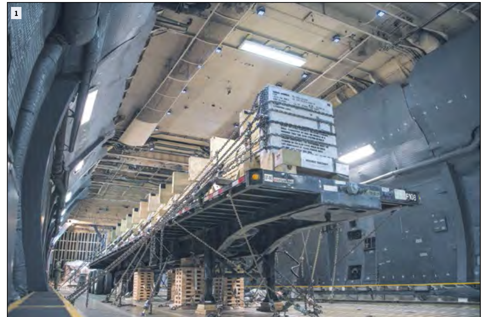
1) A U.S. Navy propulsion shaft is secured for transportation to the Pacific theater in a C-5M Super Galaxy June 9 at Travis Air Force Base, Calif. As the largest aircraft in the U.S. Air Force's inventory, the C-5M Super Galaxy serves as mobility air forces primary strategic airlift platform for transporting oversized and unconventional cargo.
